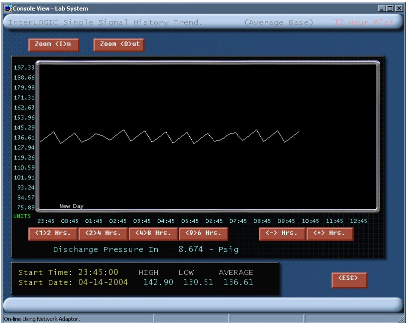
Pressing **<H>istory** on the Analog Definition Editor will display a trend graph for the selected signal. The **<+>** and **<->** buttons will go forward or back in time in 12 hour increments. Selecting one of the hours buttons, example **<2>4 Hours**, will display a trend with a total span of 24 hours. The hours buttons may be selected by pressing 1 for 12 hours, 2 for 24 hours, 4 for 48 hours and 9 for 96 hours.
