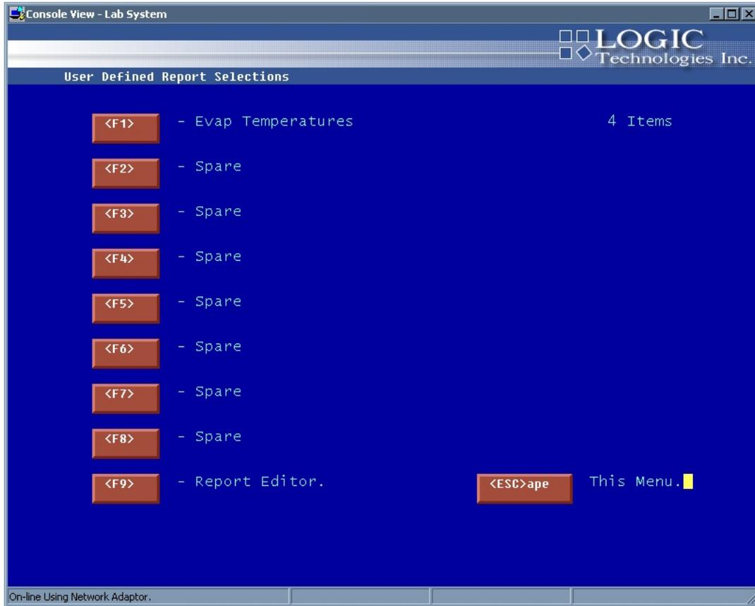
The Signal Server also allows operators to define reports to display hourly readings for a sensor point and the high, low and average reading for the day. As these report are defined, the heading will be displayed on each of the 1 to 8 selections.
