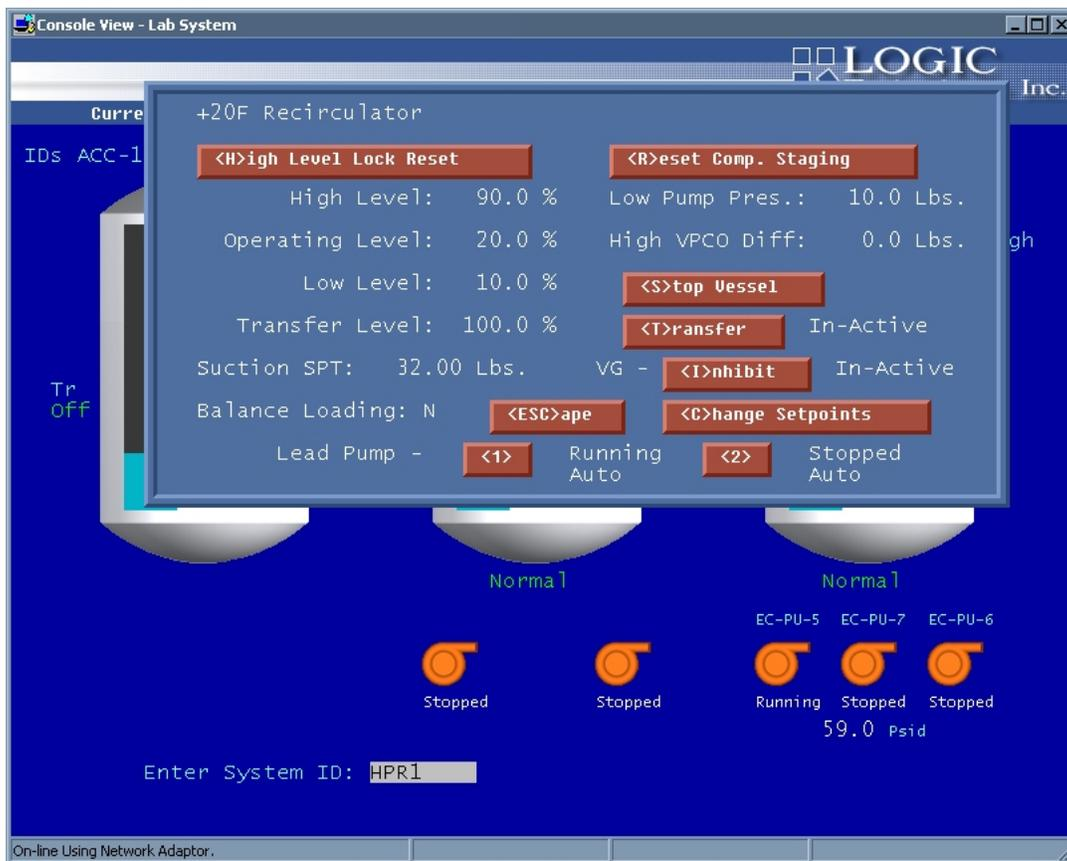
When selecting a pressure vessel to change setpoints, various modes of the setpoint window will be displayed. The vessel setup database defines the type of vessel and each type will not require the same settings. The first example on SCR-016 show the setpoint screen for a recirculator package with a variable level transmitter. The above screen is for a recirculator with float controls.
