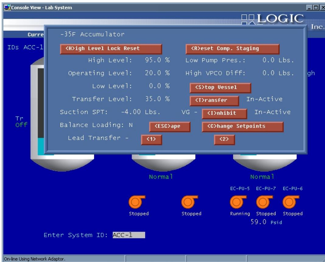
An accumulator vessel, as displayed above, may include transfer vessels to move the refrigerant liquid to a higher pressure vessel. This is accomplished using a trigger float or variable level indicator. The setpoint screen will ask for tank level trip points.
