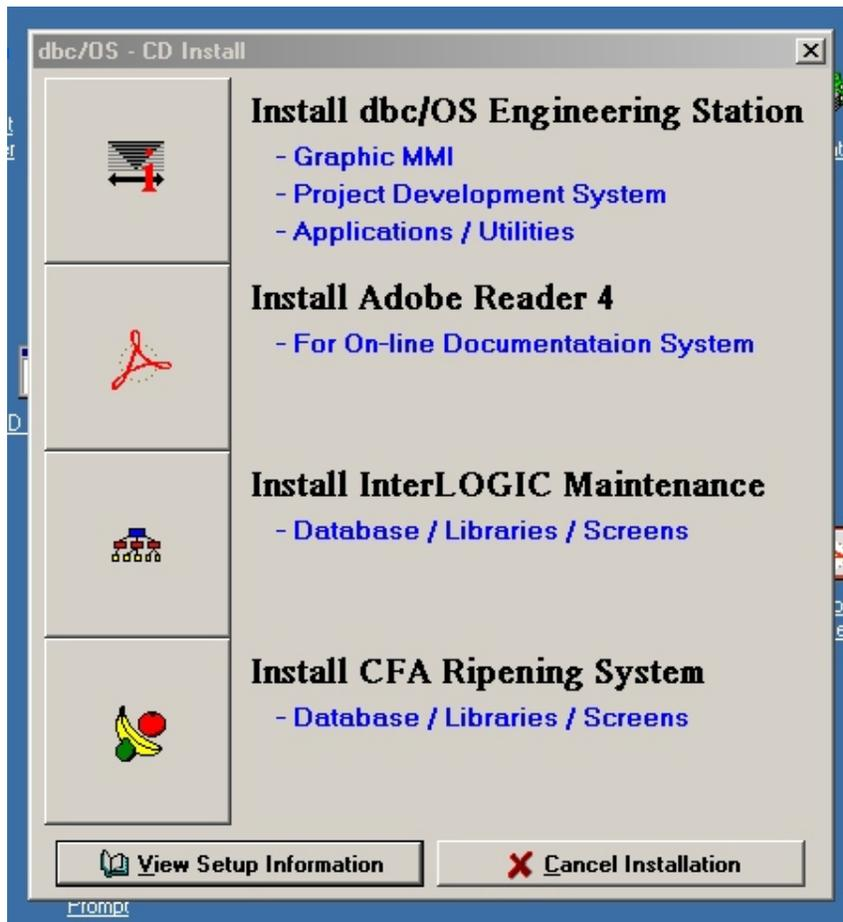
The dbc/OS Engineering Console is released on CD due to the large volume of program files installed. Setup of the software is accomplished by inserting the CD and selecting the INSTALL program located in the root directory. Upon execution of the program, the above dialog box will appear. Select the top button and when asked for install options, select custom to install all programs. If you are updating from an older version of this software, you should select the normal installation procedure.
