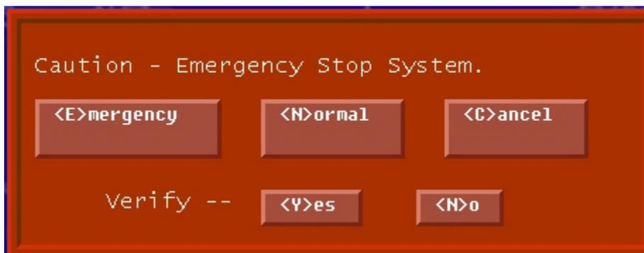
This screen will appear if the operator decides to restart the control system. This window is displayed only if selection <3> on the main screen displays "Restart System". Answering <Y>es will slowly restart the system. This will allow the engine room and air units to restage while not overloading electrical systems.
