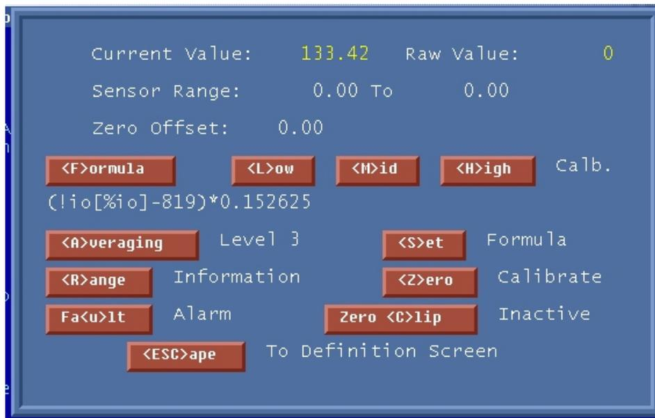
When **<L>ow**, **<M>id**, **<H>igh**, or **<Z>ero** are pressed the **Cur. Value:** prompt is displayed. The current value of the signal should be read from a known calibration source and entered at this prompt.
