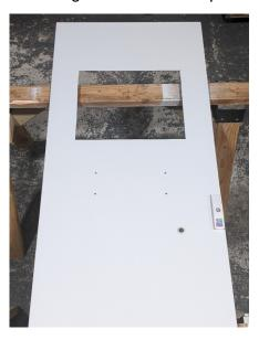
Step 5: Use A Metal File to Smooth Rough Edges of Cutout and Hole For Keyboard Wire
